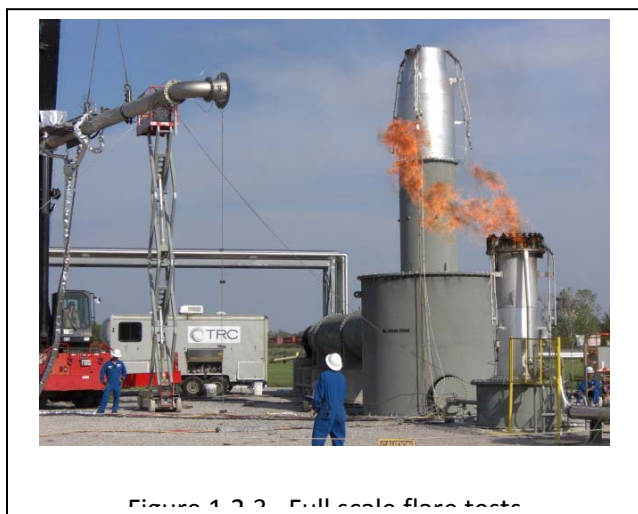
Figure 1.2.2 Full scale flare tests
