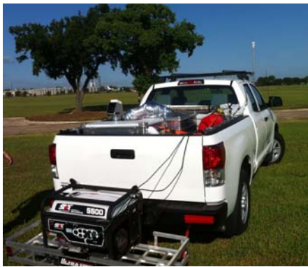
Figure 1. SOF and mobile DOAS system installed in a Toyota Tundra, here parked outside the Ellington field on Media day. Sep 2.
