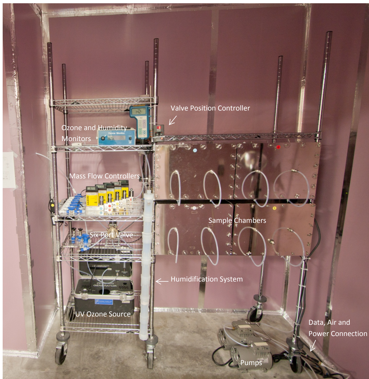
Figure 1. Digital image of the experimental system used to characterize ozone reactions with built environment surfaces.
