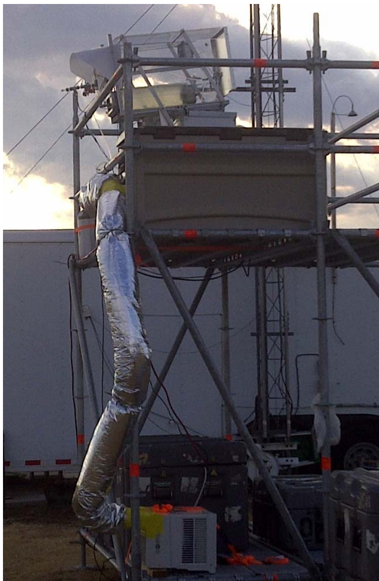
Figure 6. Close up of the MOPS instrument installed at Fort Worth Northwest (C13) site with auto-zeroing cover in the closed (zeroing) position.
