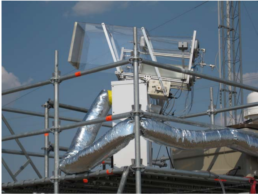
Figure 4. Close up photo of the MOPS instrument installed at Eagle Mountain Lake (C75) showing the cover zeroing mechanism.
