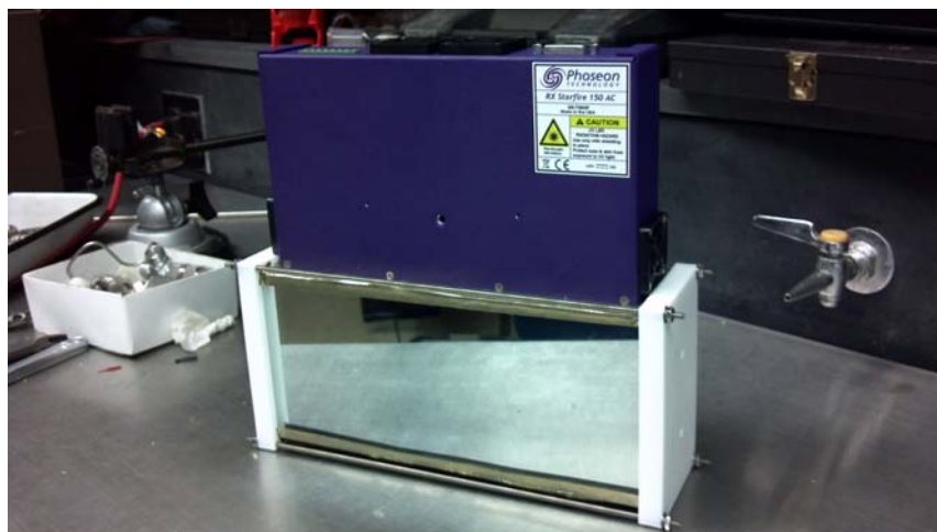
Figure 2. Photograph of the NO 2 conversion cell. In this cell a high powered LED Ultraviolet radiation source (blue) is interfaced to a polished aluminum box which contains two quartz tubes, one for each MOPS chamber (shaded and unshaded).
