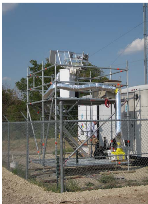
Figure 3. The MOPS instrument installed at Eagle Mountain Lake (C75). This photo shows MOPS zeroing cover in the normally open (non-zeroing) position.
