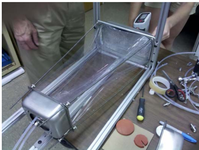
Figure 1. Photograph of the 2 nd Generation MOPS chamber. Note the coated stainless steel screen at the chamber inlet to which a temperature gradient is applied to maintain a stable boundary layer and minimize wall reactions. Photo shows leak testing of evacuated chamber with compressed walls.
