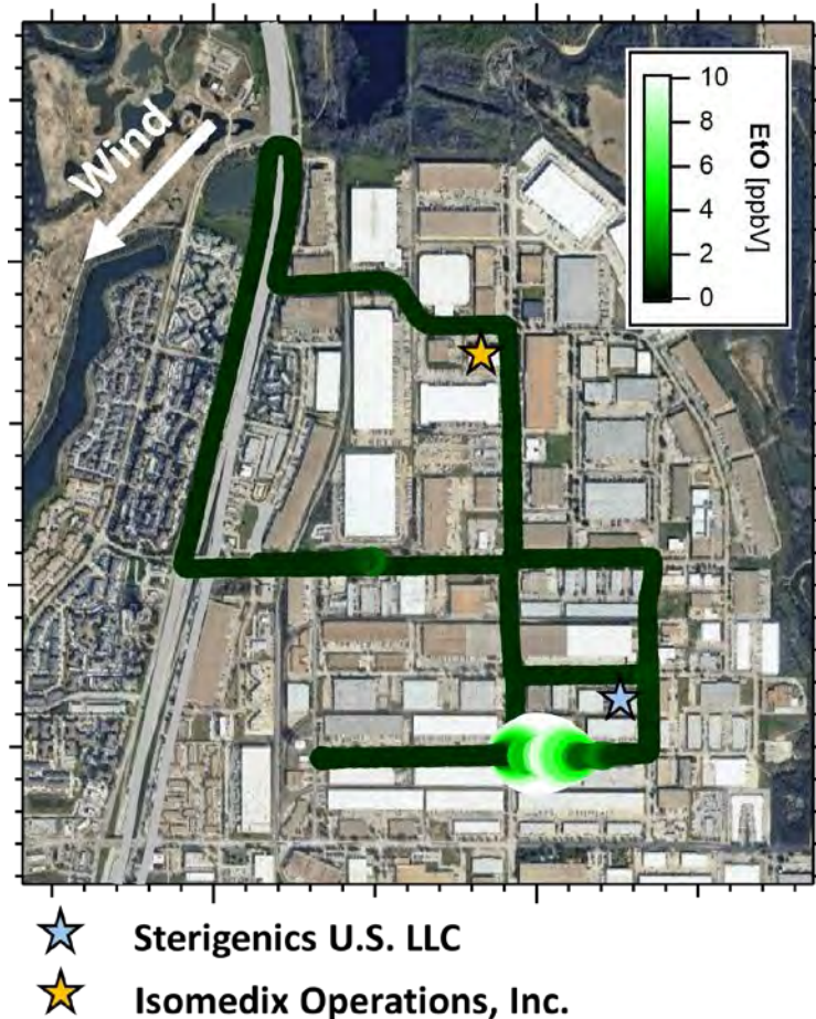
Figure 18. Mapping of ethylene oxide concentrations observed during mobile sampling between 18:15 – 18:45 UTC in the Great Southwest Industrial District of Grand Prairie, Texas, on April 6, 2023.
