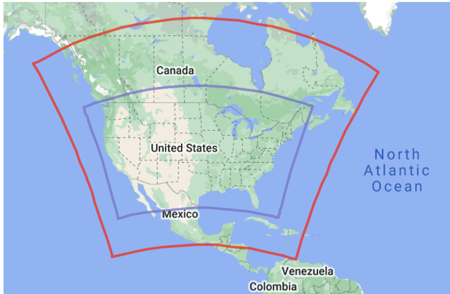
Figure 2. CAMx North American domain (red) with 36 km x 36 km horizontal resolution and nested CONUS domain (blue) with 12 km x 12 km horizontal resolution. (Source: https://www.tceq.texas.gov/airquality/airmod/data/rh/domain )
