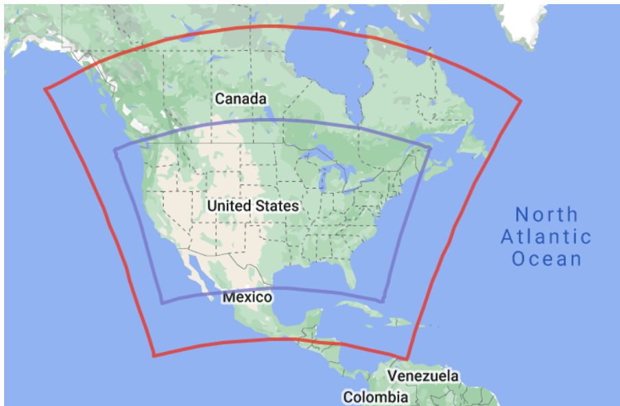
Figure 1.1. CAMx North American domain (red) with 36 km x 36 km horizontal resolution and nested CONUS domain (blue) with 12 km x 12 km horizontal resolution. (Source: https://www.tceq.texas.gov/airquality/airmod/data/rh/domain )
