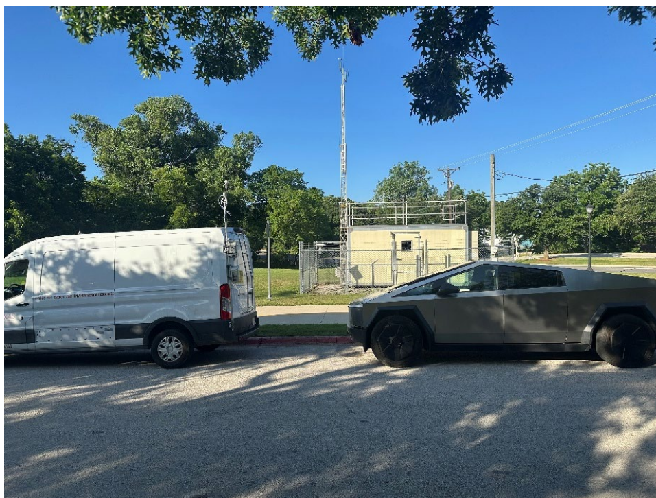
Figure 12. Stationary collocation at the TCEQ monitoring site near the University of Texas at Arlington (32.72611°N, 97.10833°W). The UT Sniffer Van and the TAMU Cybertruck-towed trailer were co-located alongside the TCEQ CAMS shelter under ambient conditions.
